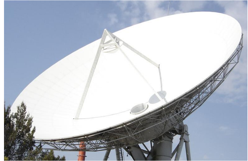
Figure 15.31 Gregorian reflector arrangement and its equivalent surface.
