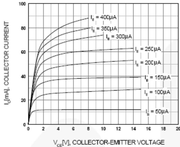
Figure 1. Static Characteristic
