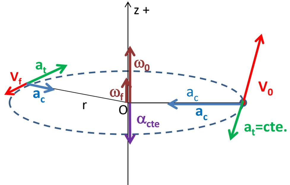
$$\omega_f = \omega_0 - \alpha \cdot (t_f - t_0) \quad V_f = V_0 + a_t \cdot (t_f - t_0)$$
