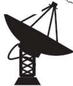
(a) Parabolic dish antenna (continuous aperture)
