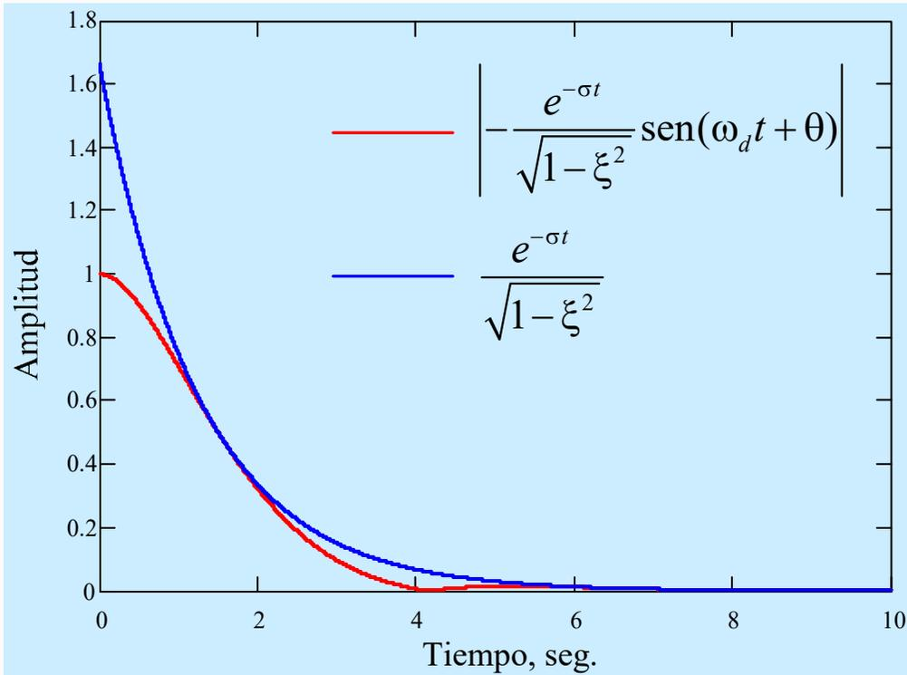
$$D := |y(t) - 1| = \left| -\frac{\omega_n}{\omega_d} e^{-\sigma t} \text{sen}(\omega_d t + \theta) \right| \leq \frac{\omega_n}{\omega_d} e^{-\sigma t} = \frac{e^{-\sigma t}}{\sqrt{1-\xi^2}}$$
