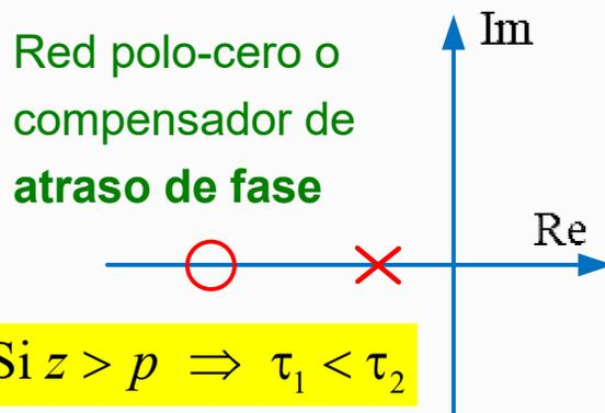
donde:  $T = R_1 C_1$ ;  $\beta T = R_2 C_2$
