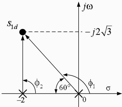
$$\left. \begin{aligned} \angle \frac{4}{s(s+2)} \Big|_{s=s_{1d}} &= -\phi_1 - \phi_2 = -(180^\circ - 60^\circ) - 90^\circ \\ \phi_{planta} &= -210^\circ \end{aligned} \right\}$$
