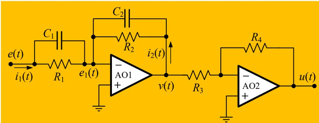
$$\tau_1 = T = R_1 C_1 \text{ y } \tau_2 = \alpha T = R_2 C_2$$
