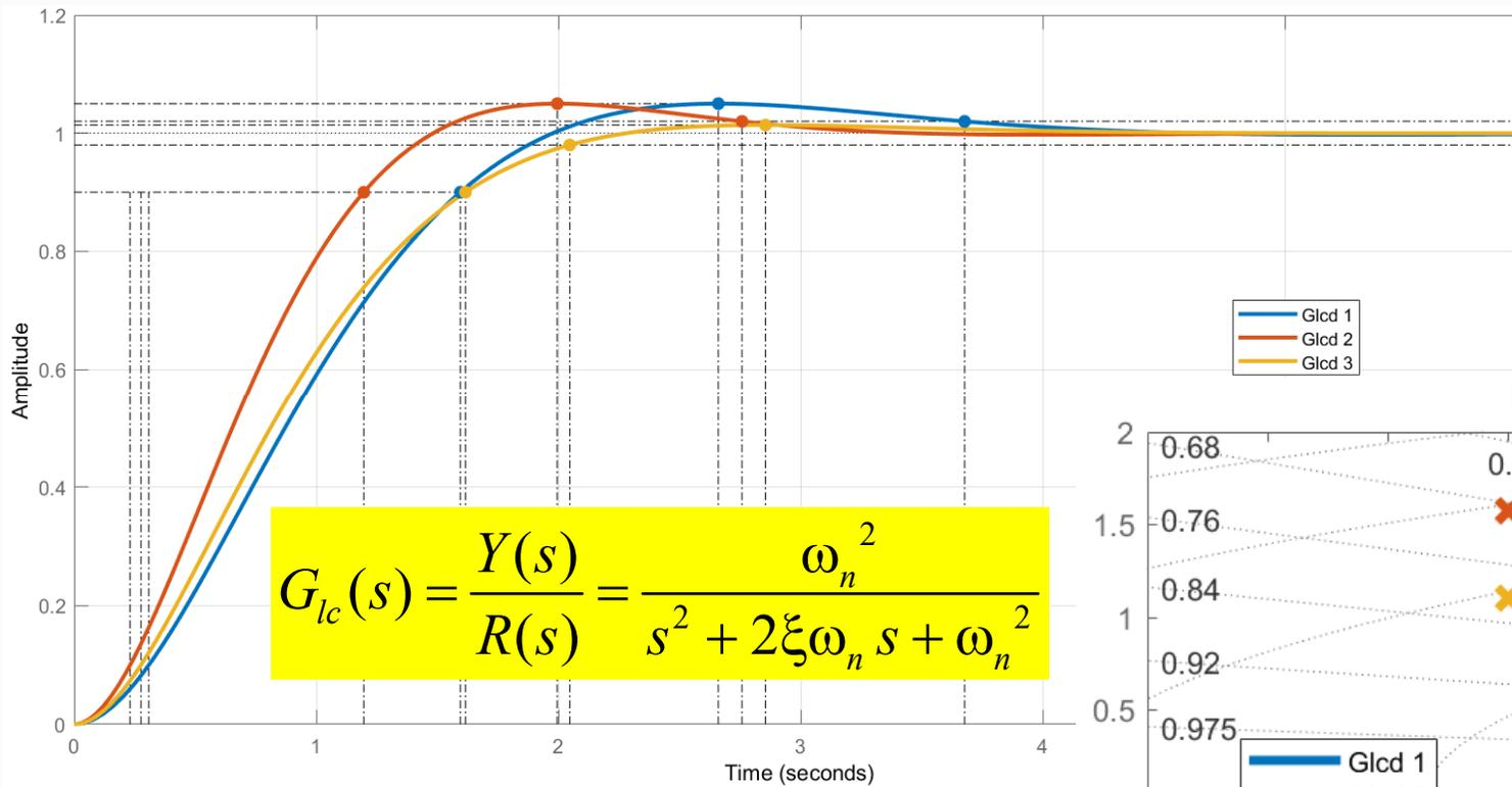
$$G_{lc}(s) = \frac{Y(s)}{R(s)} = \frac{\omega_n^2}{s^2 + 2\xi\omega_n s + \omega_n^2}$$
