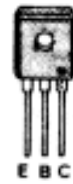
BD137 NPN BD138 PNP BD139 NPN BD140 PNP MC140 NPN MC150 PNP
