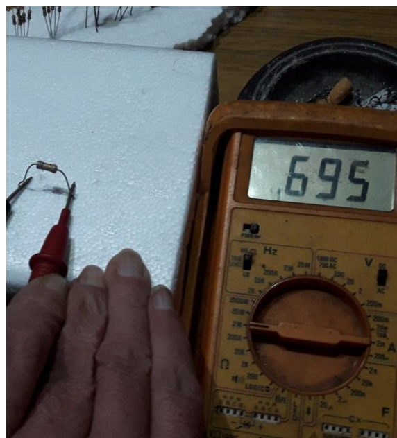
Fig 1.b: Correcto – R_{NOMINAL} = 680\text{ k}\Omega
