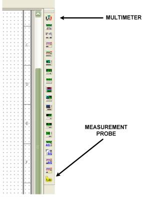
Attach the measurement probe to node 2 and then attach the multimeter across nodes 2 and 0 as shown next
