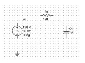
To wire up the circuit, we can left click on one component terminal, hold down, and drag the connection to a second terminal, then left click a second time. You may also connect from a component terminal to an existing circuit path. The completed circuit is then as shown
