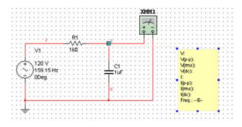
We've repositioned the probe output window to view both conveniently. If you doubleclick the probe window, you can select its parameters and de-select everything except for the rms value. For the multimeter, make sure that it is set to AC voltage. If you then hit
