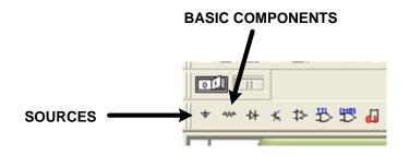
**NOTE EVERY CIRCUIT IN MULTISIM MUST HAVE A GROUND NODE**. The GROUND element is located in the SOURCES library. The voltage source is found in the POWER\_SOURCES sub-library (as AC\_POWER). The resistor and capacitor can be most conveniently specified by using the BASIC – BASIC VIRTUAL sub-library and selecting RESISTOR\_VIRTUAL and CAPACITOR\_VIRTUAL (as these components enable us to assign arbitrary values). Drag and drop these components onto the sheet.
