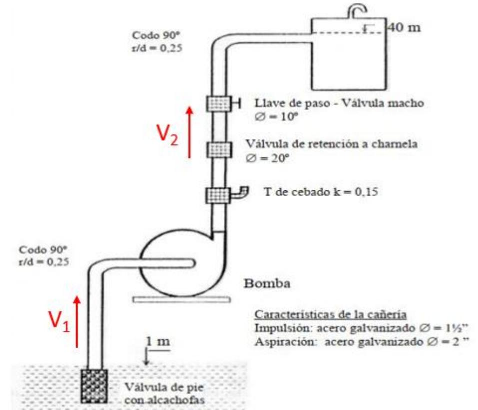
$$H_{rt} = 0,028 \frac{(4m + 0,9m + 3m) (1,37m/s)^2}{0,0508m} \frac{1}{2 \cdot 9,81m/s^2} + 0,028 \frac{(32m + 0,9m + 2,1,6m + 0,22m) (2,44m/s)^2}{0,0381m} \frac{1}{2 \cdot 9,81m/s^2} \rightarrow H_{rt} = 8,9m$$
