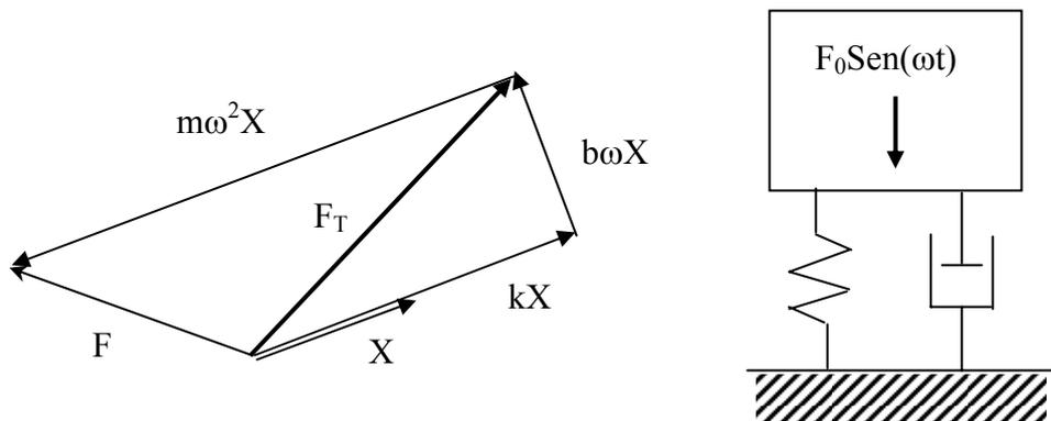
$$F_T = \sqrt{(kX)^2 + (b\omega X)^2} = kX \sqrt{1 + \left(\frac{b\omega}{k}\right)^2}$$
