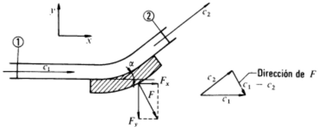
$$\begin{aligned}c_{1x} &= c_1, & c_{2x} &= c_2 \cos \alpha \\c_{1y} &= 0, & c_{2y} &= c_2 \sin \alpha\end{aligned}$$
