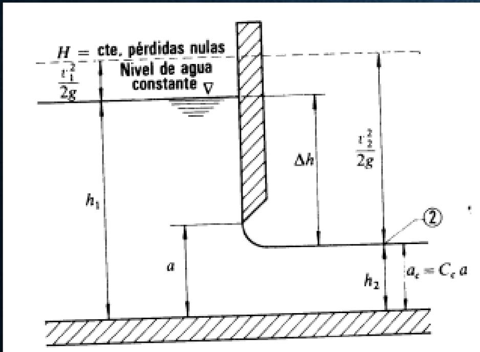
$$\frac{p_1}{\gamma} + \frac{v_1^2}{2 \cdot g} + h_1 = \frac{p_2}{\gamma} + \frac{v_2^2}{2 \cdot g} + h_2$$
