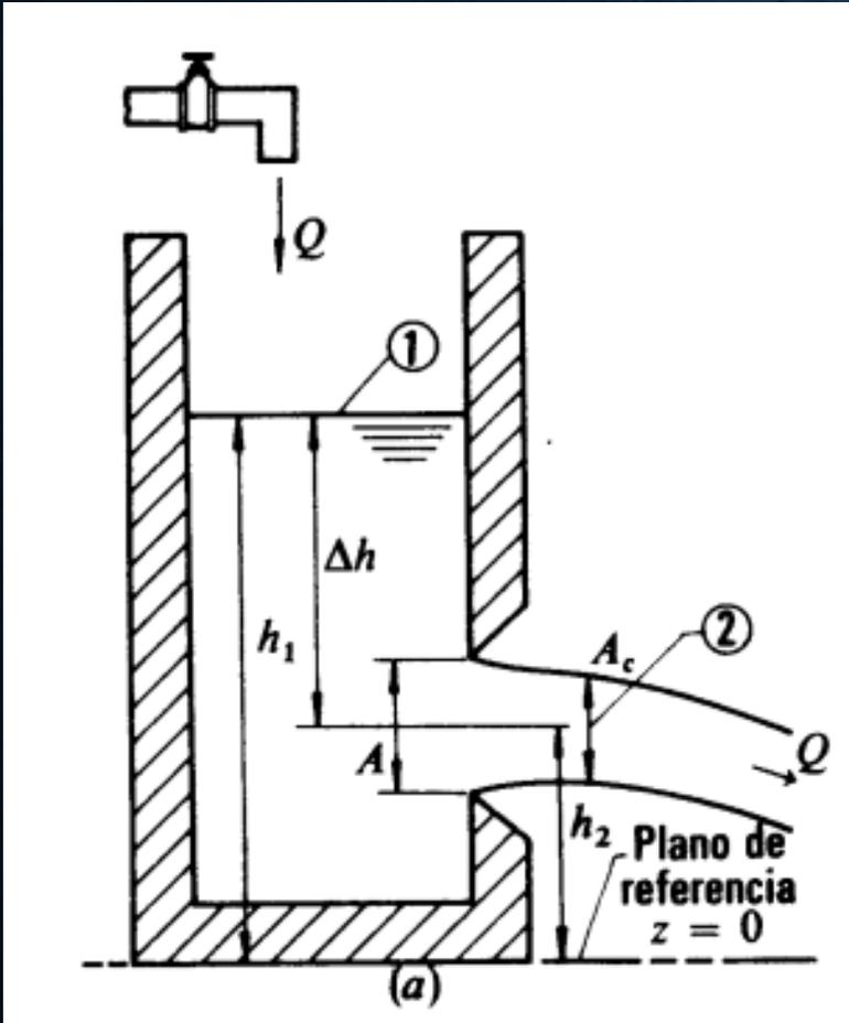
$$\frac{p_1}{\gamma} + \frac{v_1^2}{2 \cdot g} + h_1 = \frac{p_2}{\gamma} + \frac{v_2^2}{2 \cdot g} + h_2$$
