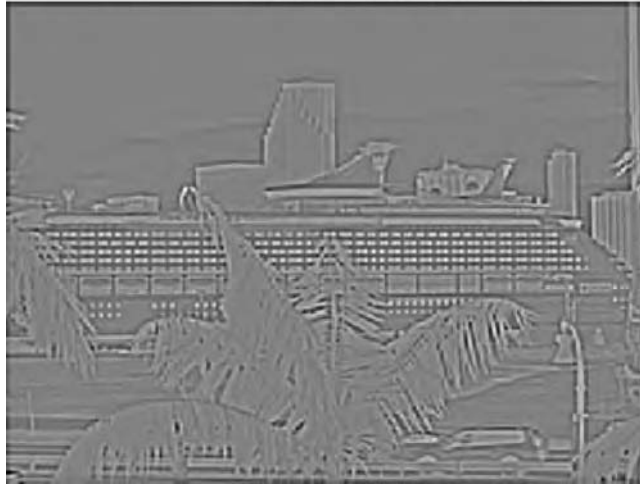
FIGURE 13.30 Image edge detection using Laplacian of Gaussian filter.
