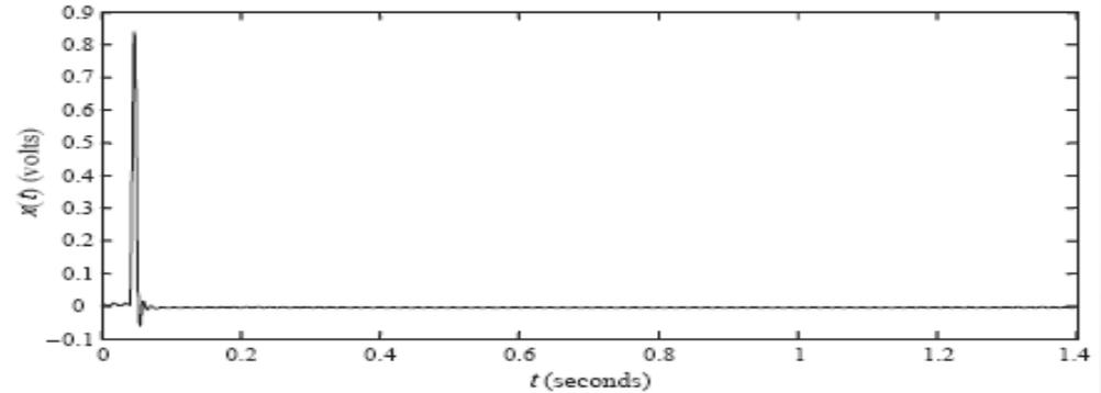
(a) Impact signal measured from the force sensor (impact hammer)
