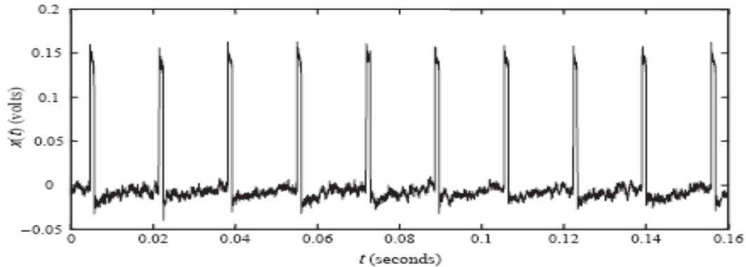
(a) Tachometer signal from a rotating machine
