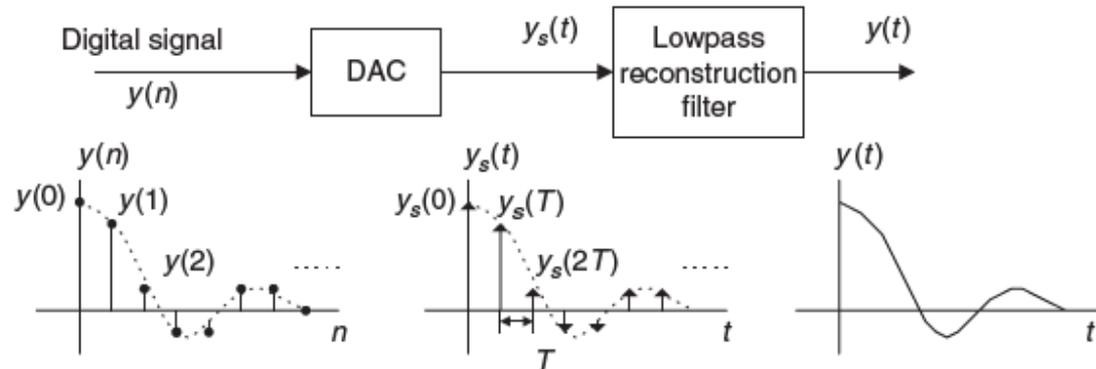
A Digital signal processed    B Sampled signal recovered    C Analog signal recovered
