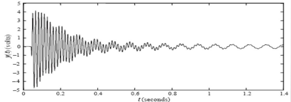
(b) Response signal to the impact measured from the accelerometer
