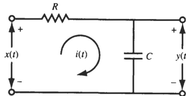
$$H(\omega) = \frac{Y(\omega)}{X(\omega)} = \frac{1}{1 + j\omega RC} = \frac{1}{1 + j\omega/\omega_0}$$
