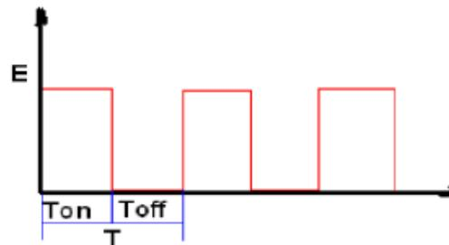
$$V_{med} = E \times \frac{T_{on}}{T}$$
