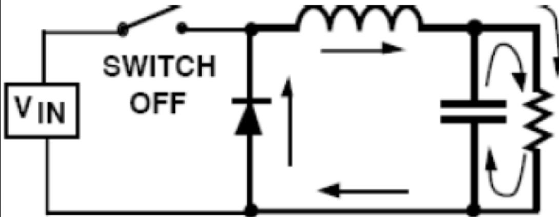
$$i_l(off) = i_{pk} - \frac{V_{out}}{L} T_{off}$$
